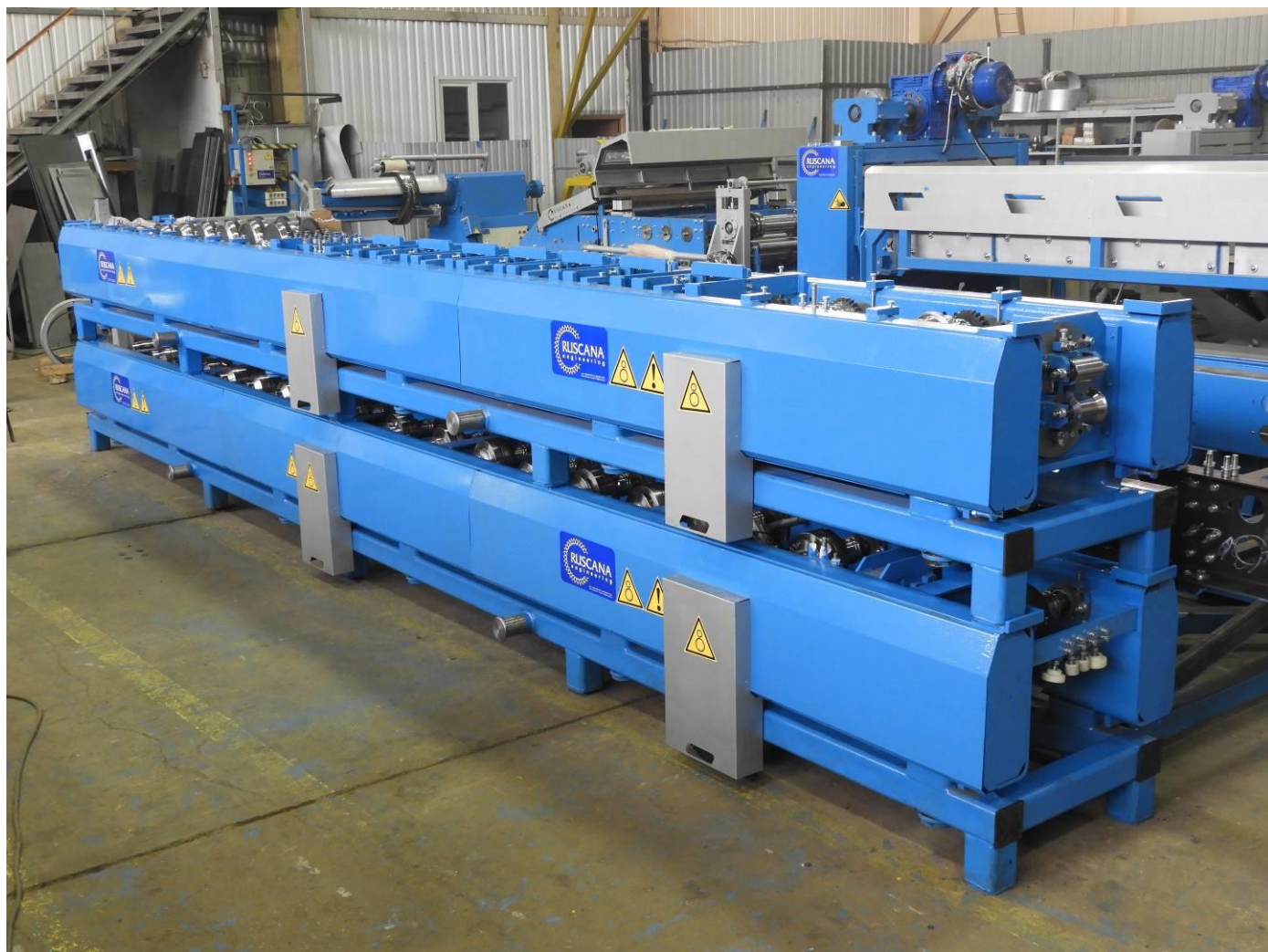
Fig. 2 Roll forming cassettes
