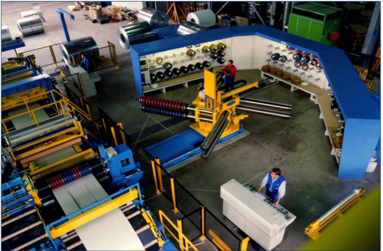
Fig. 14. An example of organizing a metal sheet slitting section
