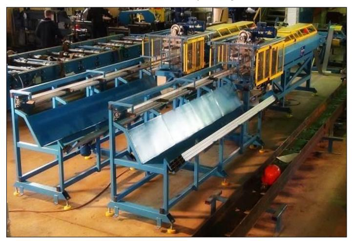
*U channel 28x27 roll forming line*, hereinafter referred to as Equipment, is intended for producing profiles for wall partitions and suspended ceilings. See profile drawing fig.1
